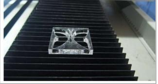
Oxidized Aluminum Knife worktable with drawer Black oxidized Aluminum alloy tool section are efficient to decrease the laser's reflecting, suitable for hard materials, such as wood, acrylic, etc.
